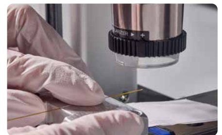
Microscopic inspection of emitter tip to confirm tip angle and tip diameter
