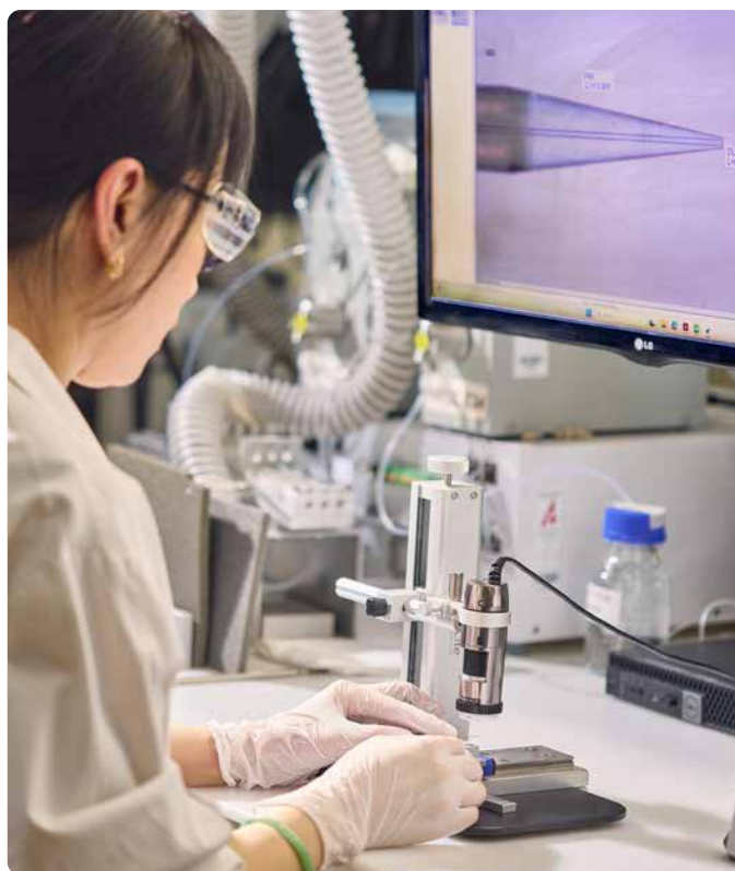
The constant bore is inspected for particulates; the geometry of the tip is also checked.
